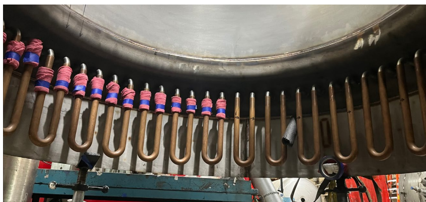
Figure 7. Photo of the copper tubes composing the 2K heat exchanger
