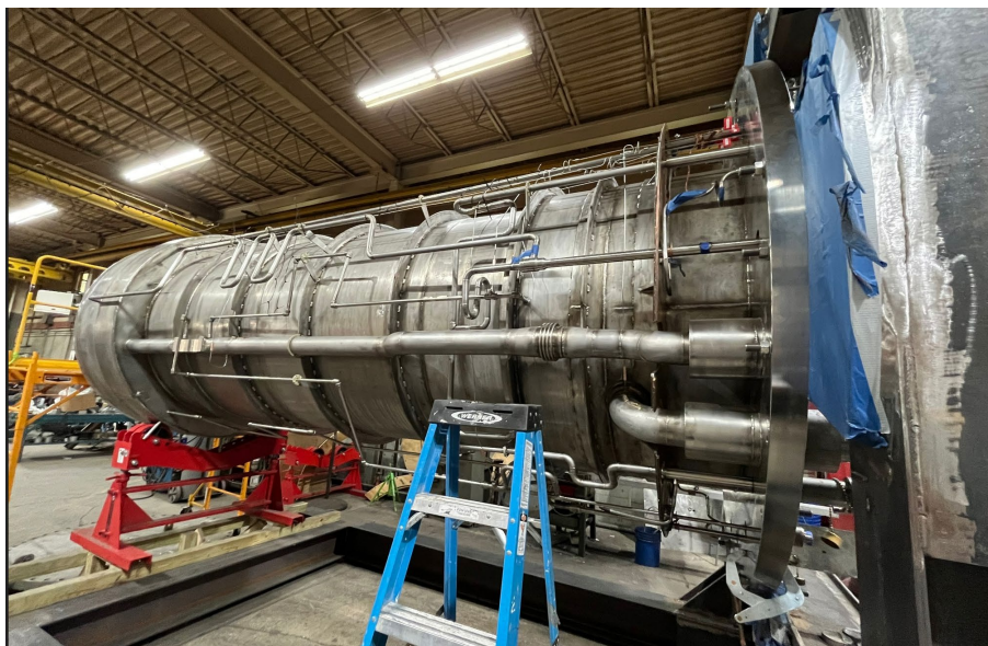
Figure 6. Photo of the helium vessel horizontal and attached to its support during fabrication
